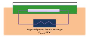
**Fig. 10.** Sketch of the ground exchanger used to limit overheating in summer and reach targeted operating range in winter. Heat exchanges were obtained by circulating water in the closed loop, between one heat exchanger immersed in the culture medium and another heat exchanger buried in the ground sand.
