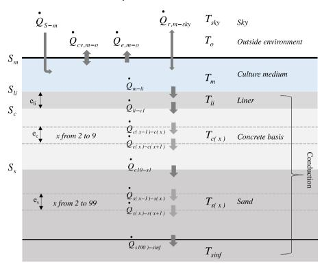
Fig. 2. Heat exchanges used in the thermal model.
