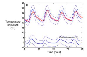
Fig. 3. Thermal model validation. Panel 3-a presents operating conditions in terms of total radiation q (solid line) and ambient temperature (dashed line) (Qatar, May 2016). Panel 3-b gives predictions of time-course change in culture temperature (solid line) and comparison to experimental measurements (dotted line). Because of the uncertainty on input data, simulations were also run assuming a deviation of  $\pm$  40% on both relative humidity and windspeed (dashed lines).
