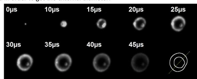
SCF+400 $\mu\text{m}$  of paint: Vaporization profile
