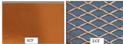
Figure 3 Lightning Strike Protection principle
