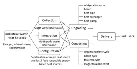
Fig. 1. The diagram of industrial waste heat recovery.
