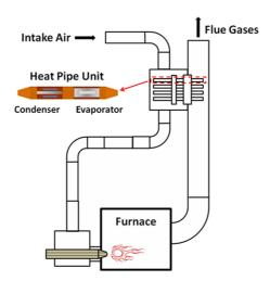
Fig. 2. Waste heat recovery using heat pipes [39].
