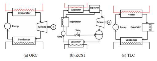
Fig. 3. Schematic diagram for basic power cycles.
