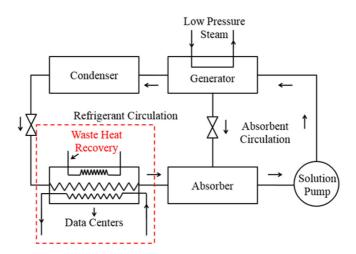
Fig. 4. Schematic of absorption refrigeration with waste heat recovery [71].
