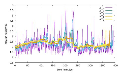
**Figure 8.** Effect of averaging duration on the electric field level — Orange LTE 800 —  $\Delta T_1 = 60$  s,  $\Delta T_2 = 360$  s,  $\Delta T_3 = 720$  s,  $\Delta T_4 = 1800$  s,  $\Delta T_5 = 3600$  s  $- Z_{\text{direct}}$ .
