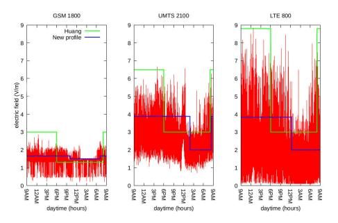
Figure 7. Time dependant exposure to an Orange base station during 24 hours.
