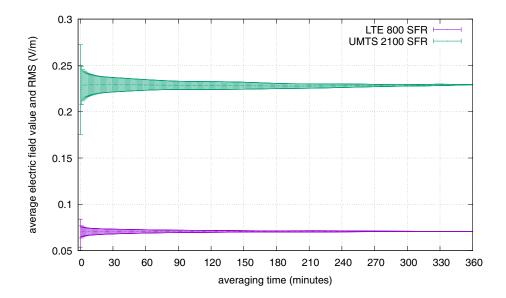
**Figure 10.**  $ES_{\Delta T}$  according to technologies for SFR in  $Z_{\text{reflection}}$ .
