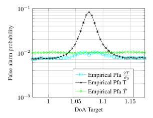
**Fig. 3**. Empirical Pfa as a function of the DoA for  $\frac{2T}{\vartheta_0}$ , T and  $\tilde{T}$ .  $M=80,\,N=80,\,K=3,\,CNR=10\,dB$ .
