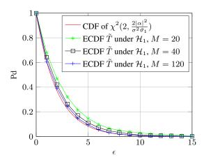
**Fig. 2.** ECDFs of  $\tilde{T}$  under  $\mathcal{H}_1$  hypothesis for different values of M and CDF of  $\chi^2(2,\frac{2|\alpha|^2}{\sigma^2\vartheta_1})$  (red).  $N=M,\,K=3,\,CNR=10dB,\,SNR=-20dB.$
