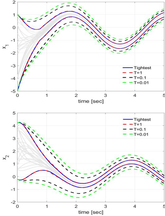
Figure 1. Comparison of open-loop interval estimators (16)-(17) for  $T = 0.01$  (green),  $T = 0.1$  (black),  $T = 1$  (red),  $T = t$  (blue). In gray are represented the state trajectories of the system generated from different initial conditions and different inputs with values on the allowed intervals.
