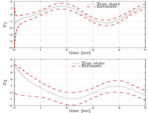
Figure 3. Closed-loop interval estimates in the scenario where the initial state  $x_0$ , the input  $w$  and the parameters are uncertain. The estimator of Theorem 12 was applied with a gain  $L = [8.685 \ -2.00]^T$  which was obtained according to the method described in Remark 3.
