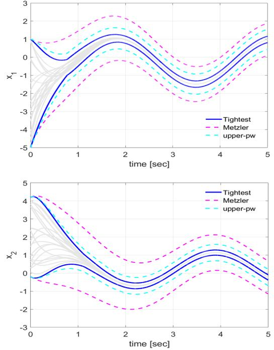
Figure 2. Comparison of open-loop interval estimators: tightest (blue), estimator (14) (cyan) obtained by upper-bounding  $p_w$  with 2, approximation using a Metzler matrix (magenta). In gray are represented the state trajectories of the system generated from different initial conditions and different inputs.
