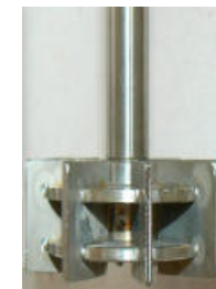
Hollow self-inducing impeller
