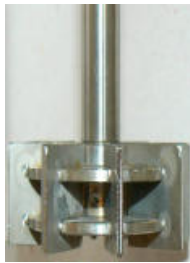
Hollow self-inducing impeller
