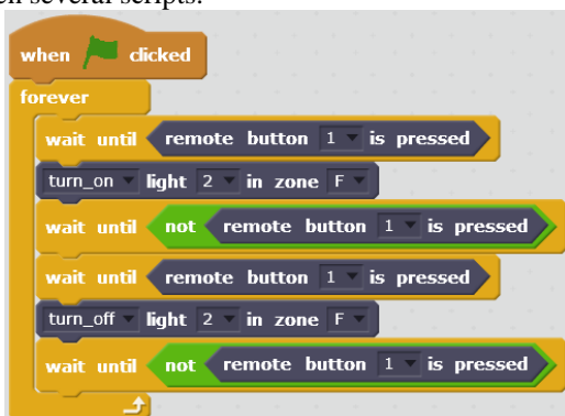
Fig. 7. Scratch 2.0 script for the light control
