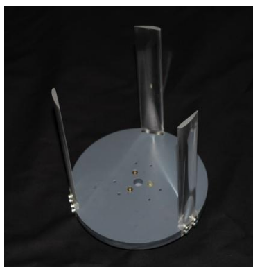
Fig 1. Vertical axis marine current turbine prototype for water channel test.
