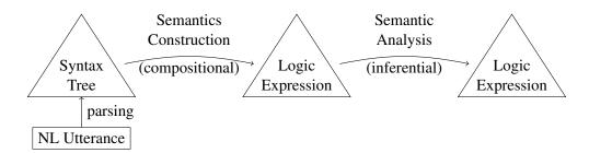
Figure 2: The pipeline of an NLU system.
