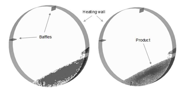
Figure 1. Simplified scheme of the drum with milli-beads distributions visualization for the bi-size bed after 8 minutes of drum rotation (24 revolutions) : on the left the small beads are black and the large ones are white, on the right the cold beads are darker and the hot ones are clearer.
