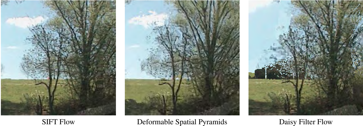
Figure 15: Image registration using SIFT Flow, Deformable Spatial Pyramids, and Daisy Filter Flow. The pixel-level alignment quality is often higher using SIFT Flow in our application.
