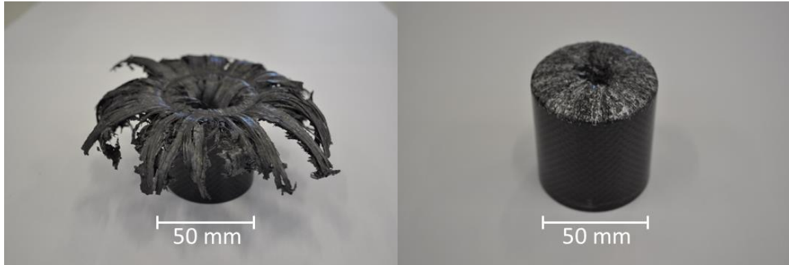
Figure 6. Crushed CFRP tubes showing outer spreading (left) and inner folding (right).
