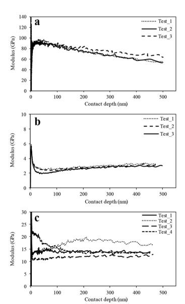
**Fig. 9.** Elastic modulus obtained by MTS indentation for (a) glass fibers, (b) PP matrix and (c) flax fibers.
