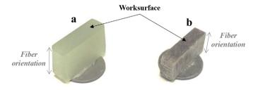
Fig. 1. a) glass/epoxy workpiece. b) flax/PP workpiece.
