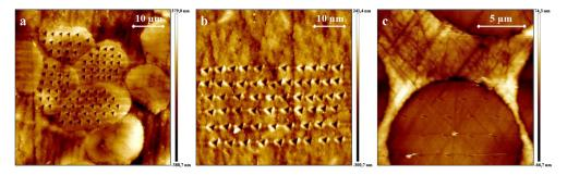
Fig. 5. Topographic AFM images after indentations for (a) flax fibers (b) PP matrix and (c) glass fiber.
