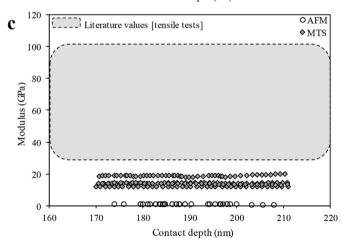
**Fig. 10.** Comparison of the elastic modulus obtained by AFM and MTS Nanoindenter with the literature results. (a) glass fiber, (b) PP matrix and (c) flax fibers.
