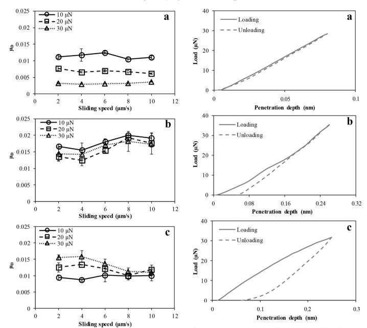
**Fig. 12.** Dynamic friction coefficient obtained by AFM scratch test for different applied loads. (a) glass fibers, (b) PP matrix and (c) flax fibers.
