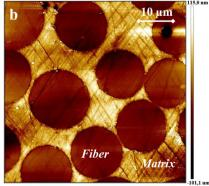
Fig. 4. Topographic AFM images before indentation for (a) flax/PP and (b) glass/epoxy.
