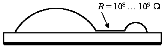
Figure 22. Schematic of a small satellite droplet connected to the reservoir drop via a thin channel. The ohmic resistance of the channel can exceed the capacitive impedance between the satellite and the bottom electrode (thick black line).
