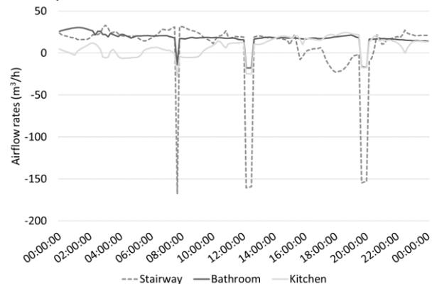
**Fig. 6.** Natural ventilation airflow rates multizone-coupled simulation.
