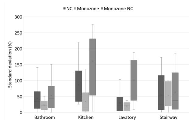
**Fig. 7.** Natural ventilation airflow rates standard deviation.
