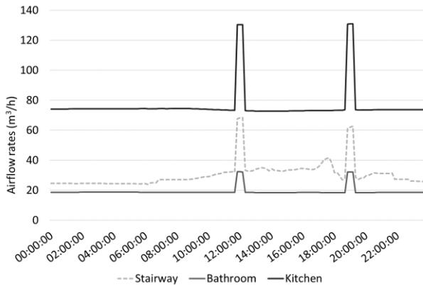
**Fig. 3.** Balanced ventilation airflow rates multizone-coupled simulation.
