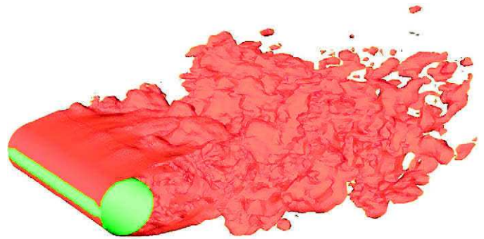
Fig. 7. Numerical simulation of single cylinder vibration under sub-critical cross flows (Jus, 2011).
