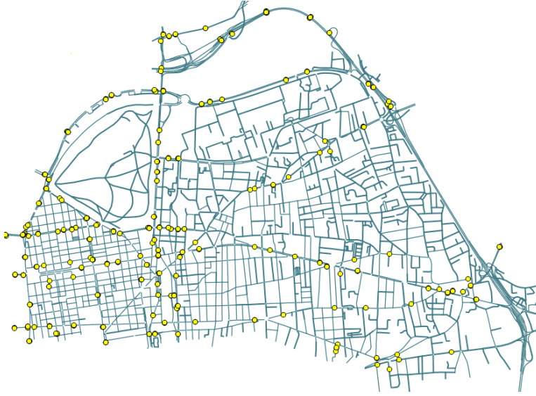
Fig. 2: The Lyon road network considered in the study, and the actual positions of sensors placed by the agglomeration of Lyon city (in yellow).
