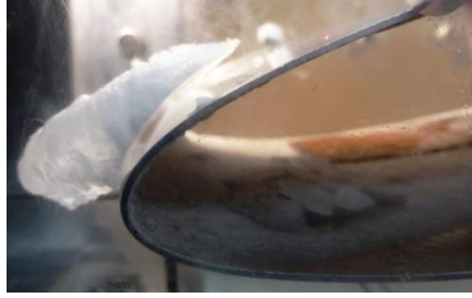
Fig. 12 – Test of the leading edge sample with thicker and rime ice excited around 31 kHz
