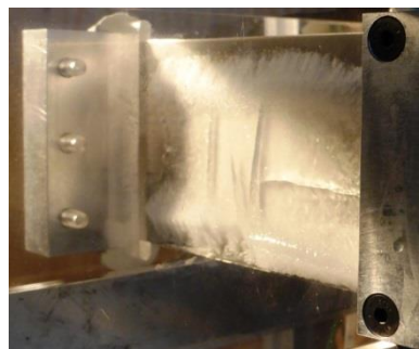
Fig. 6 – De-icing result for the test specimen C excited around 5 kHz for 90 V
