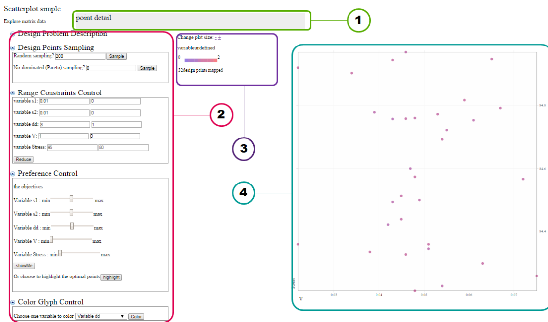
Figure 8. Screenshot of the platform interface with the four main zones. (1) Details about one design point; (2) Menu with functions; (3) Info about design space and (4) Visualization of the design space.
