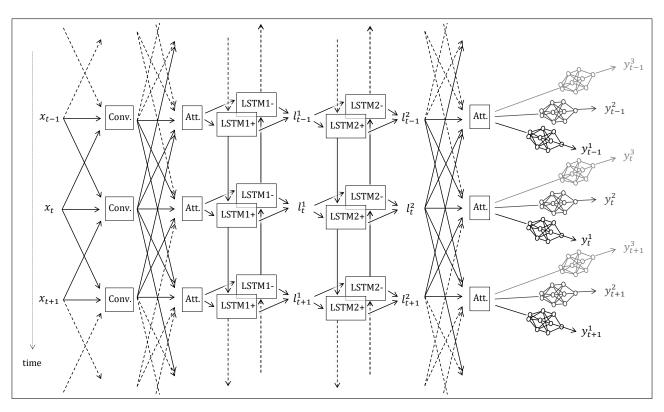
Figure 2: Simplified unfolded scheme of a RNN network for SL linguistic features learning. From left to right, the followings layers are stacked: input, 1D-convolution, attention, bidirectional LSTM  $(2\times)$ , attention, multi-layer perceptron before each output feature;
