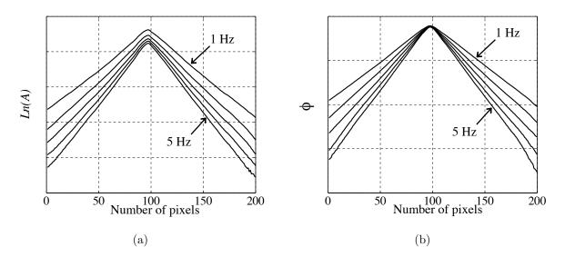
Figure 14: Profiles of amplitude (a) and phase difference (b) along a cracked minicomposite, for frequencies ranging from 1Hz to 5Hz.
