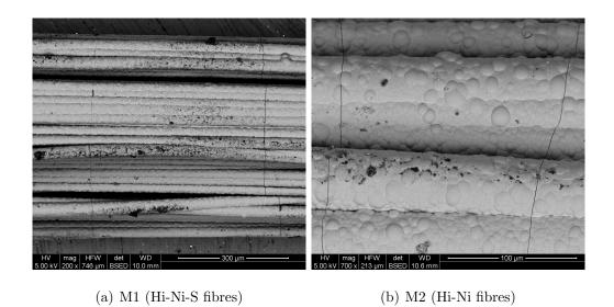
Figure 10: Scanning Electron Microscopy micrographs showing matrix cracks perpendicular to fibre direction, after minicomposite failure.
