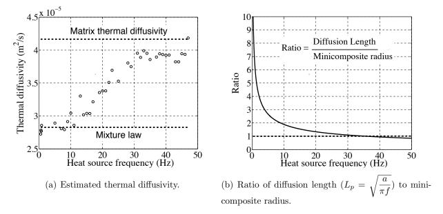
Figure 6: Results obtained from virtual testing of minicomposite. Influence of the local heat source frequency (LASER) on the estimated thermal diffusivity.
