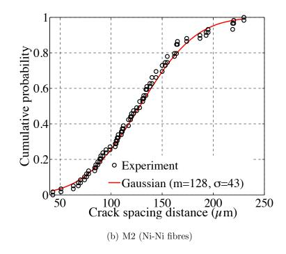
Figure 8: Statistical distribution of crack spacing distances in minicomposites (after failure) measured by Scanning Electron Microscopy.
