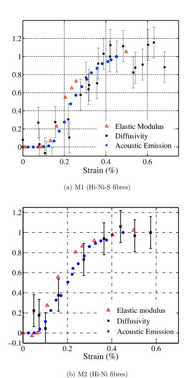
Figure 15: Comparison of damage indicators derived from elastic modulus, thermal diffusivity and acoustic emission during axial tensile tests.
