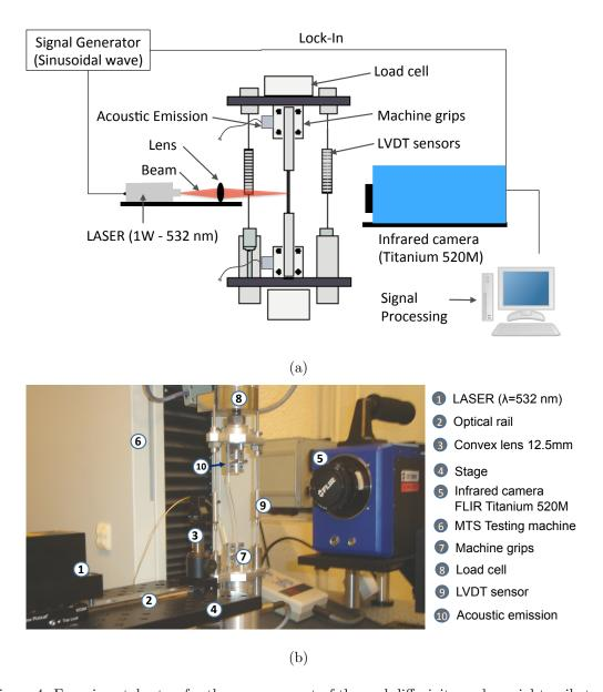
$Figure \ 4: \ Experimental \ setup \ for \ the \ measurement \ of \ thermal \ diffusivity \ under \ axial \ tensile \ test.$
