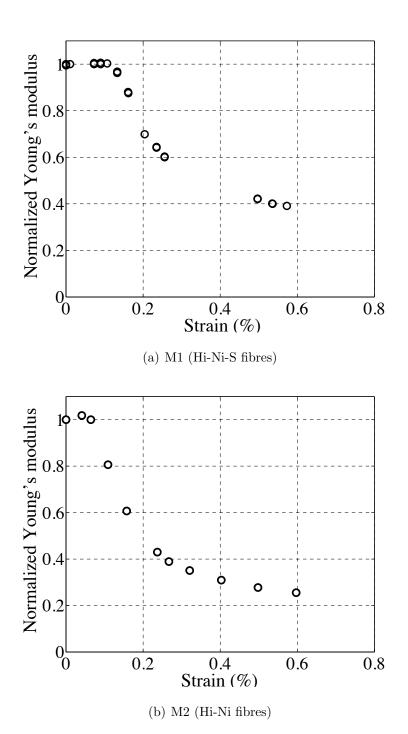
Figure 9: Degradation of Young's modulus of SiC/SiC minicomposites extracted from loading-unloading cycles during axial tensile tests.
