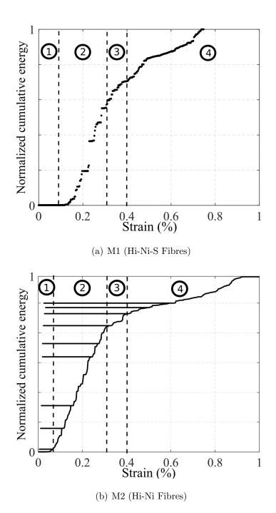
Figure 12: Dimensionless acoustic emission cumulative energy during axial tensile tests.
