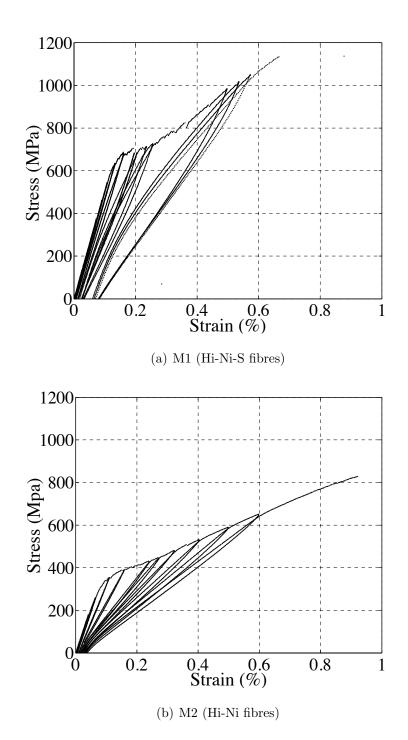
Figure 7: Tensile stress-strain curves that exhibit the features of the well-known elastic damageable behavior of SiC/SiC composites.
