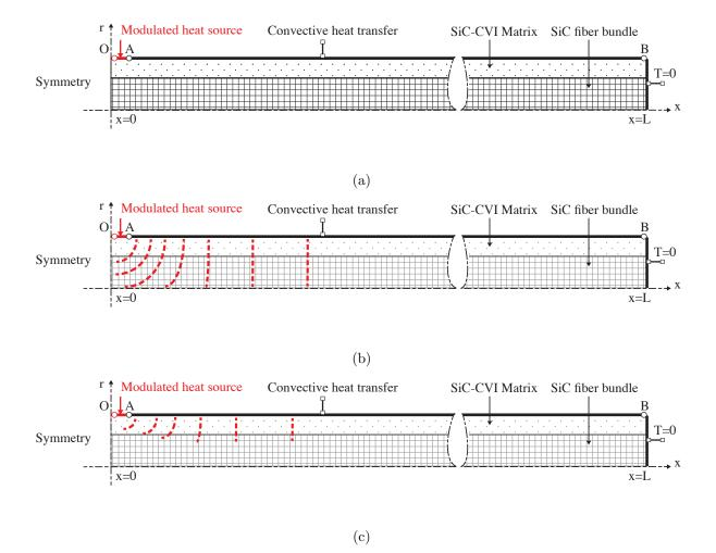
Figure 5: (a) Simplified model of minicomposite for virtual testing (thermal diffusivity measurement) using Finite Element Analysis (FLEXPDE Software). Schematic representation of isotherms for (b) frequencies smaller than 10Hz and (c) frequencies larger than 35Hz.
