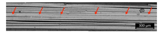
Figure 11: Scanning Electron Microscopy micrographs showing randomly distributed matrix cracks after minicomposite failure.
