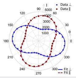
**FIG. 4**. Polar plots of intensities (I) transmitted through the optical collector and the monochromator.  $\theta$  is the analyzer angle from the horizontal position. Data are displayed as round and square markers for the transmission of  $\perp$  and  $\parallel$  polarized light at the stage, respectively. Plain lines represent a fit using a modified Malus' law that includes unpolarized light and a rotation.
