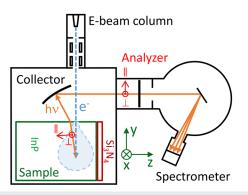
FIG. 2. Experimental setup. The optical collector is schematized.
