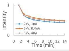
FIG. 5. Evolution of the luminescence intensity with measurement time for three e-beam settings. Intensities are normalized.
