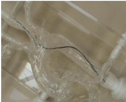
Fig. 13. Test on a silicon-based anatomical phantom
