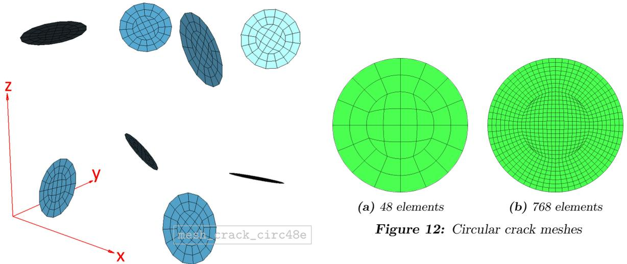
**Figure 11:**  $2 \times 2 \times 2$  crack array
