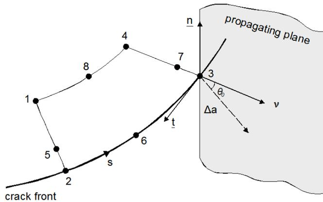
**Figure 4:** Quarter-point element at the crack front. Vectors  $\boldsymbol{\nu}, \mathbf{n}, \mathbf{t}$  constitute the local coordinate frame at node **3**. Their directions respectively correspond to the opening, sliding and tearing local modes of fracture propagation.
