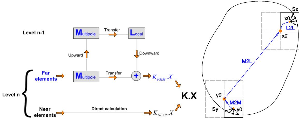
**Figure 3:** Two-level multipole algorithm (left); Multipole operations M2M, M2L and L2L (right)
