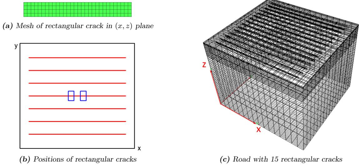
**Figure 16:** Three-layered road with multiple stationary rectangular cracks: arrangement
