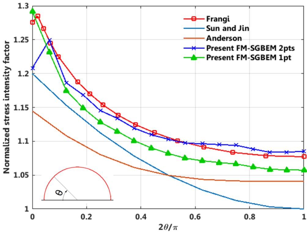
Figure 9: Surface-breaking crack: normalised SIF  $K_I^*$  along the crack front
