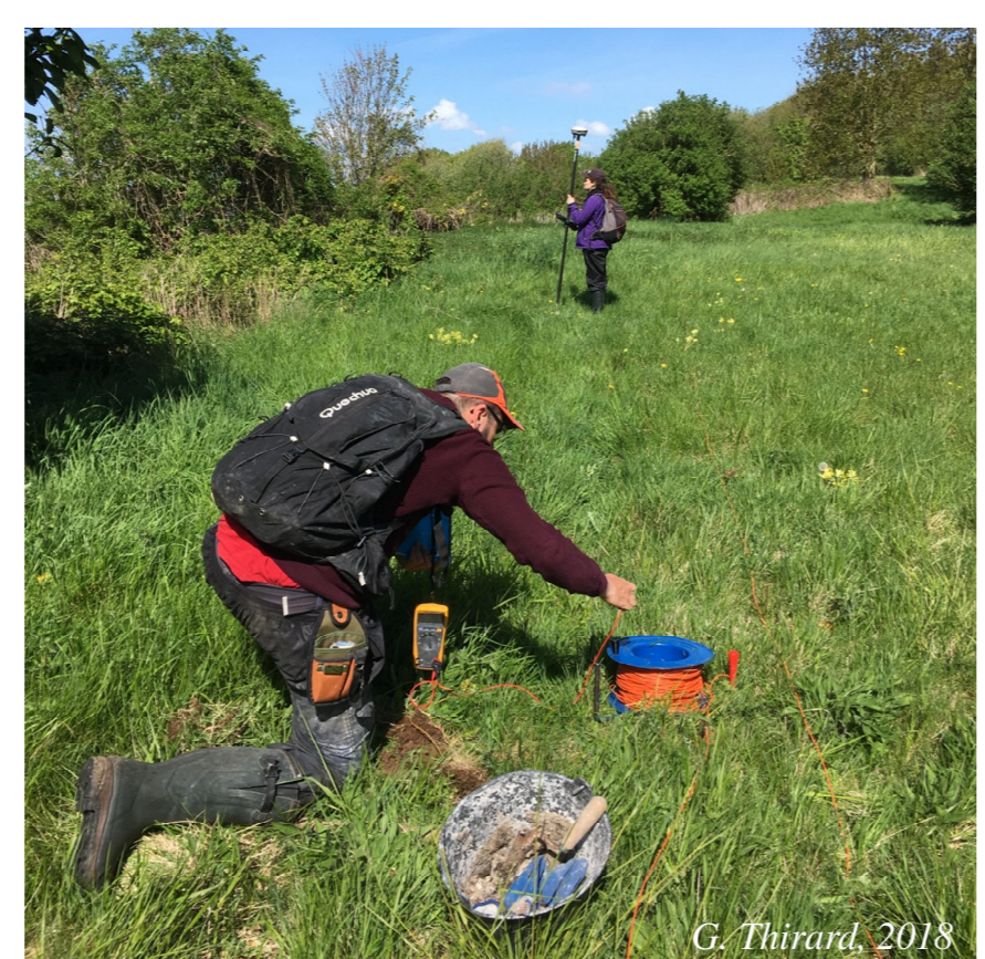
Figure 2. SP and GPS surveys during the spontaneous polarization survey
