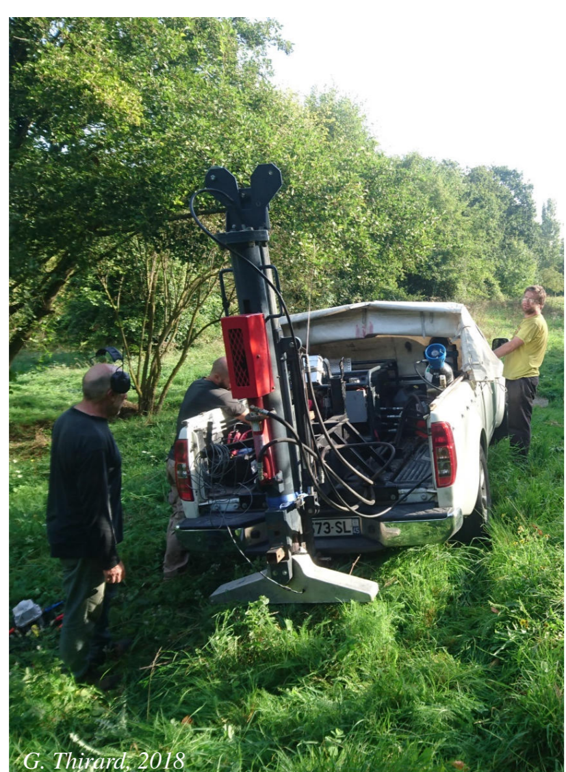
Figure 4 – Seismic in-vehicle source on the transverse profile
