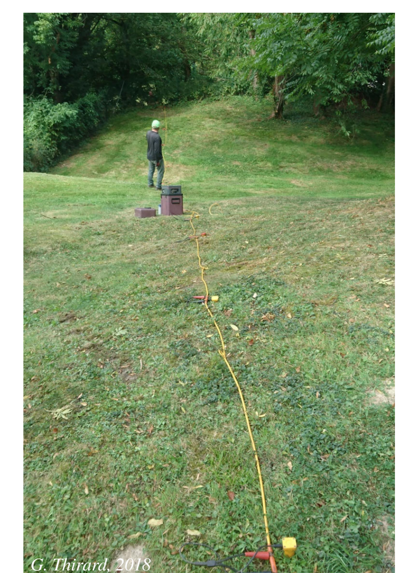
Figure 3 – Seismic streamer on the upstream-downstream profile
