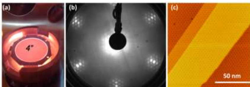
Fig. VII.1: 800 °C hot 4 inch wafer (a). Low energy electron diffraction (LEED) pattern of h-BN/Rh(111) at 60 eV kinetic energy (b). STM image of the same surface with U_t = -1.2 V and I_t = 0.5 nA.
