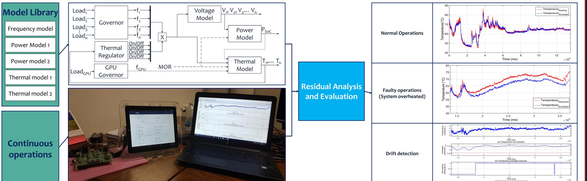
Fig 2. Interconnected and Incremental modeling and online monitoring
