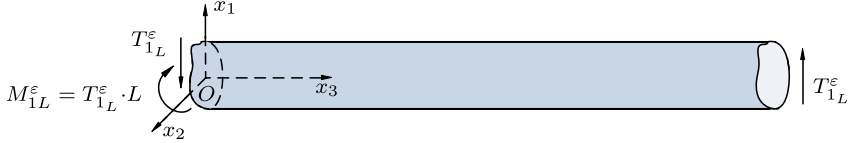
Fig. 3 Loadings applied on the prism (simple bending)
