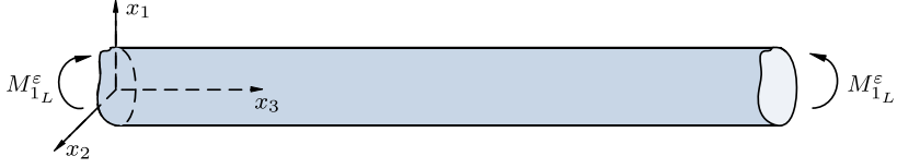
Fig. 2 Loadings applied on the prism (pure bending)
