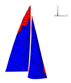
Figure 20. Sign of Vx for the "inviscid optimum" trim computed with ARA-ISIS
