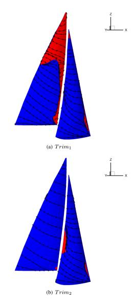
Figure 7. Sign of Vx computed with ARA-ISIS Blue surfaces show the direct flow and red surfaces show the reverse flow.
