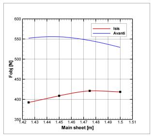
Figure 19. Optimum trim (main car fixed at 0.2m)
