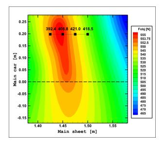
Figure 18. Optimum trim Negatives values: windward side Positives values: leeward side
