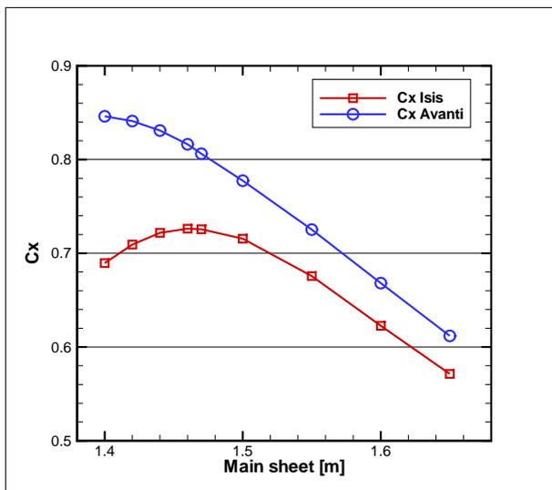
Figure 3.  $C_x$  versus the main sheet length
