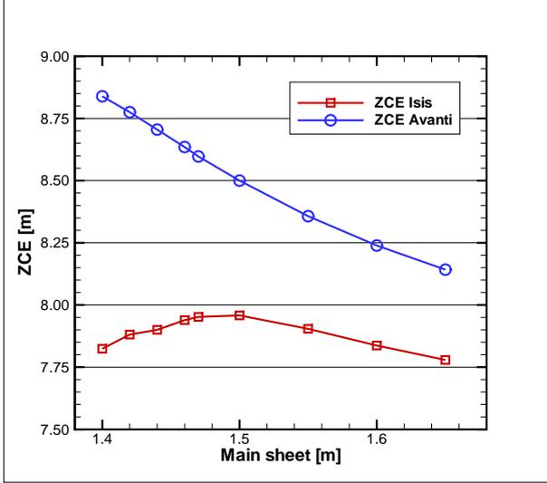
Figure 6. ZCE versus the main sheet length
