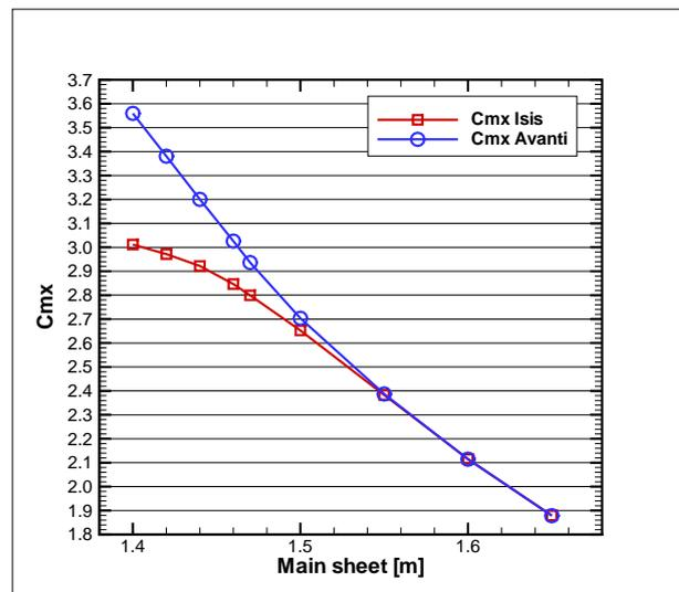
Figure 5.  $C_{mx}$  versus the main sheet length
