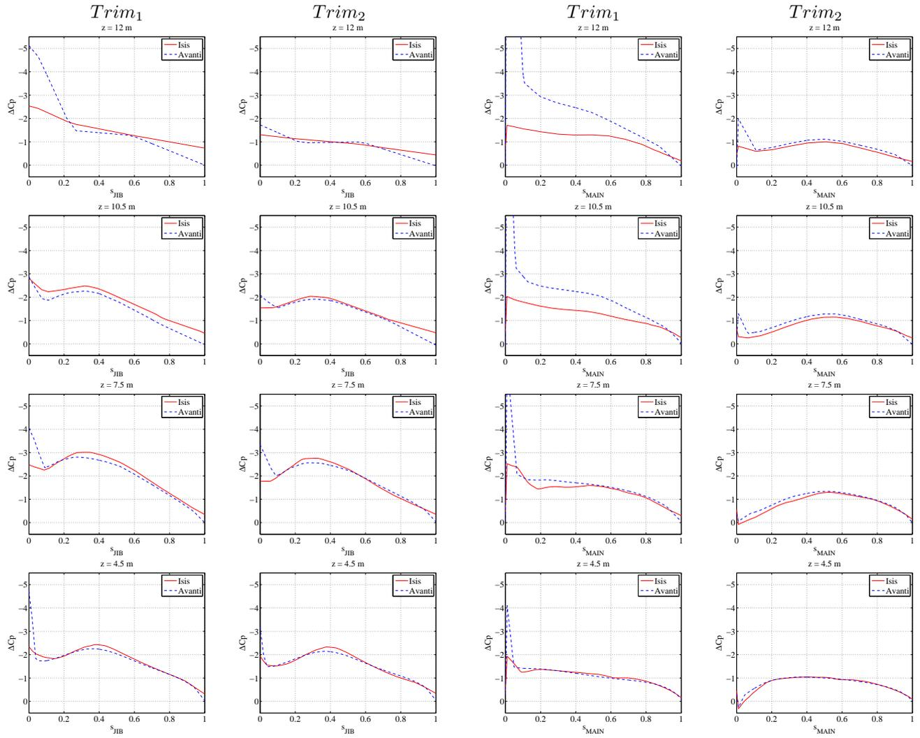
**Figure 8. Jib  $\Delta C_P$  along the height**
