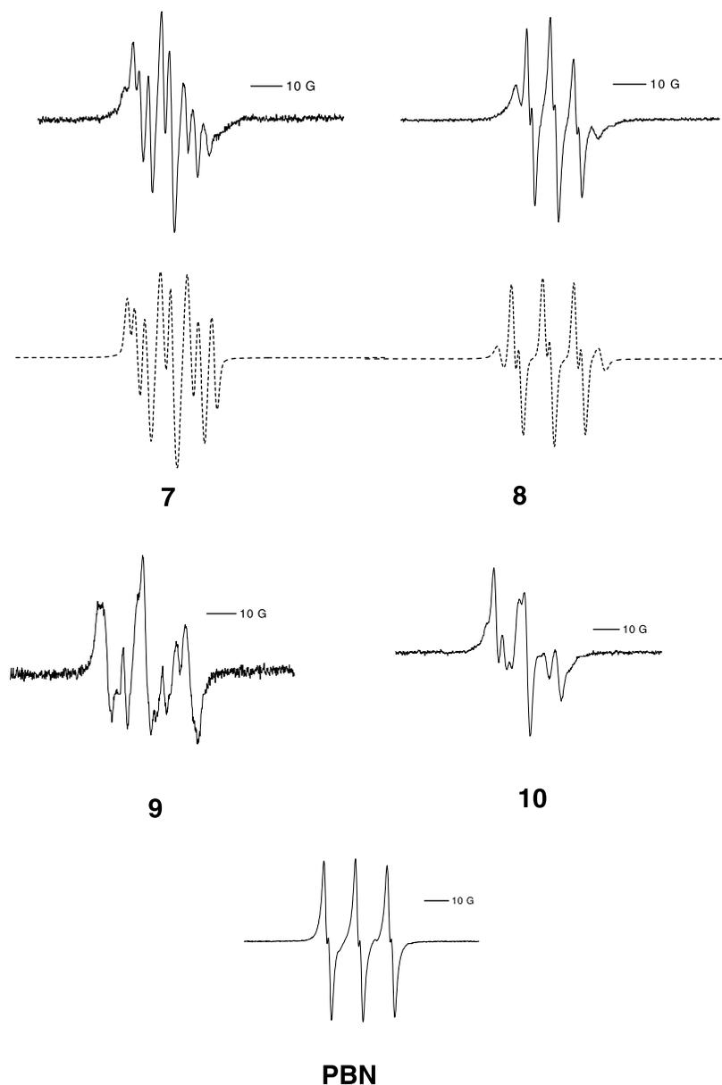
Figure 5. EPR spectra of nitrones **1–10** and PBN (10 mM) with  $\text{CH}_3 \cdot \text{CH} \cdot \text{CH}_3$  prepared in benzene from isobutyric acid and lead tetraacetate (45/45 mM). Gain:  $5.64 \times 10^3$ . Solid lines: experimental spectra; dashed lines: simulated spectra.
