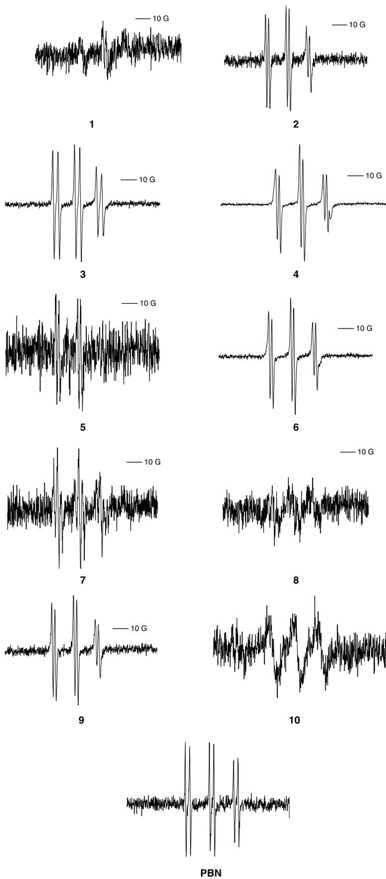
Figure 4. EPR spectra of nitrones **1-10** and PBN (10 mM) with  $\cdot\text{CH}_3$  generated by Fenton's reaction ( $\text{Fe}^{2+}/\text{H}_2\text{O}_2$ :100/100  $\mu\text{M}$ ) in  $\text{H}_2\text{O}/\text{DMSO}/\text{DMF}$ : 30/60/10 (v/v). Gain:  $5.64 \times 10^4$ .
