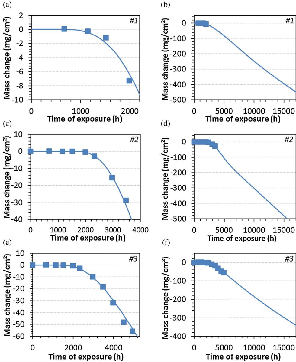
**Fig. 14.** Experimental net mass changes (squares) and mass losses modelled using Model II (curve) for samples (a and b) #1, (c and d) #2 and (e and f) #3 in  $\text{H}_2\text{-CO-CO}_2\text{-CH}_4\text{-H}_2\text{O}$  at  $570^\circ\text{C}$ , 21 bar.
