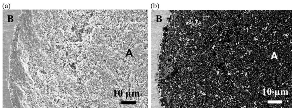
**Fig. 4.** (a) SE and (b) BSE SEM pictures of a pit containing corrosion products (noted A) and the oxide scale at its edges (noted B) after 1987 h in  $\text{H}_2\text{-CO-CO}_2\text{-CH}_4\text{-H}_2\text{O}$  at  $570^\circ\text{C}$ , 21 bar.
