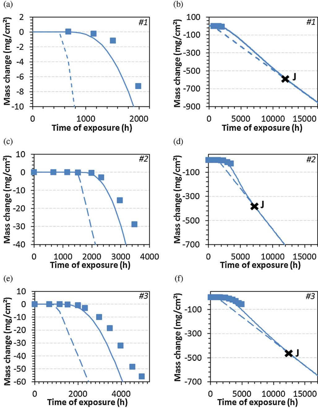
**Fig. 15.** Experimental net mass changes (squares) and mass losses modelled using Model III (continuous curve) and Model IV (dashed line) for samples (a and b) #1, (c and d) #2 and (e and f) #3 in  $H_2-CO-CO_2-CH_4-H_2O$  at 570 °C, 21 bar.
