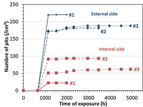
**Fig. 5.** Evolution of the number of pits on external (blue diamonds) and internal (red squares) side of 800HT samples #1 (continuous line), #2 (dashed line) and #3 (dotted line) in  $\text{H}_2\text{-CO-CO}_2\text{-CH}_4\text{-H}_2\text{O}$  at  $570^\circ\text{C}$ , 21 bar. (For interpretation of the references to color in this figure legend, the reader is referred to the web version of this article.)
