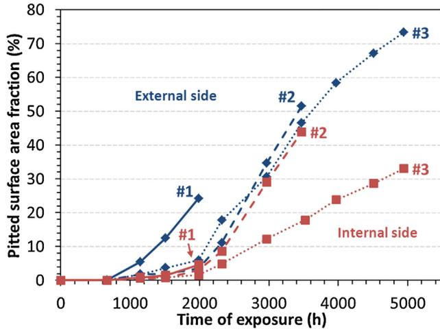
**Fig. 7.** Evolution of the pitted surface area fraction for external (blue diamond) and internal (red squares) sides of 800HT samples #1 (continuous line), #2 (dashed line) and #3 (dotted line) in  $H_2$ -CO-CO<sub>2</sub>-CH<sub>4</sub>-H<sub>2</sub>O at 570 °C, 21 bar. (For interpretation of the references to color in this figure legend, the reader is referred to the web version of this article.)
