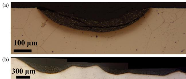
**Fig. 8.** (a) Cross section of etched sample #1 after 1987 h of exposure in  $H_2$ -CO-CO<sub>2</sub>-CH<sub>4</sub>-H<sub>2</sub>O at 570 °C, 21 bar. (b) Overlapping between pits after 4941 h for sample #3.
