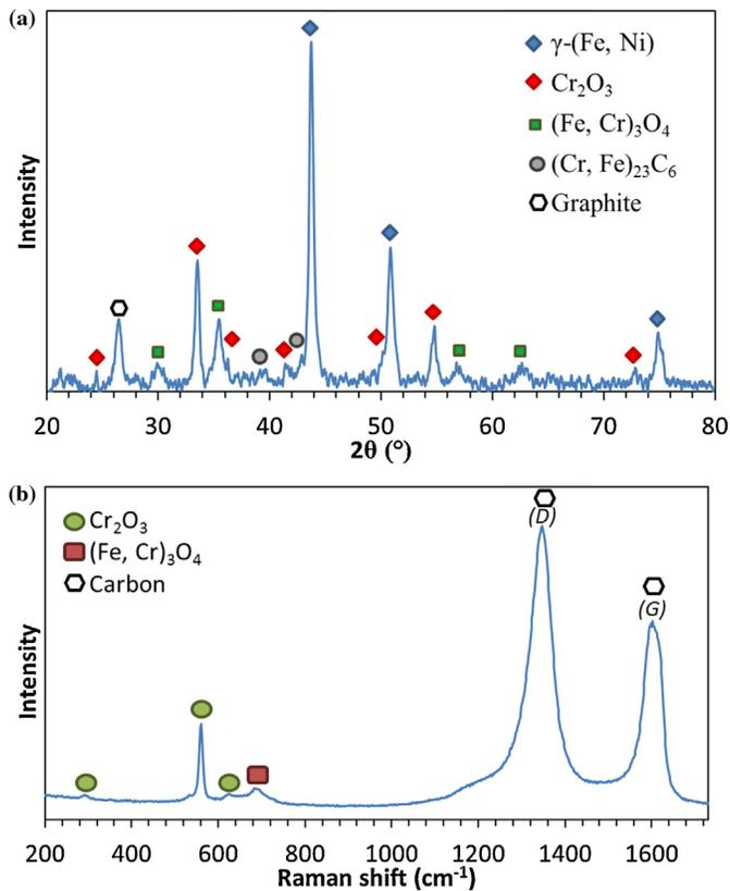
**Fig. 3.** (a) XRD and (b) Raman spectra of 800HT sample #1 after 1987 h in  $\text{H}_2\text{-CO-CO}_2\text{-CH}_4\text{-H}_2\text{O}$  at  $570^\circ\text{C}$ , 21 bar. (D) and (G) represent signals for disordered and ordered carbon, respectively.
