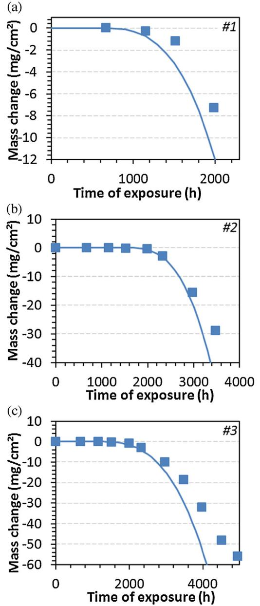
Fig. 13. Experimental net mass changes (squares) and mass losses modelled by Model I (continuous curve) for samples (a) #1, (b) #2 and (c) #3 in  $\text{H}_2\text{-CO-CO}_2\text{-CH}_4\text{-H}_2\text{O}$  at 570 °C, 21 bar.
