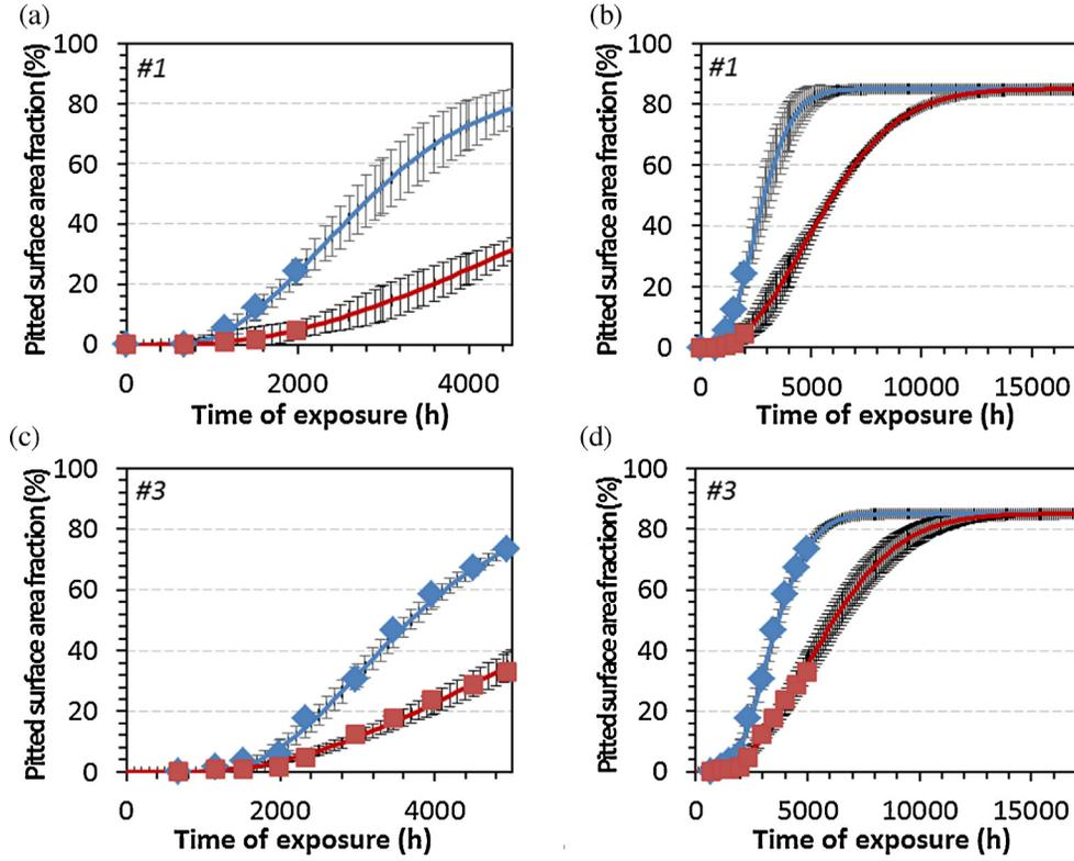
**Fig. 11.** Experimental (symbols) and calculated (curves) pitted fraction area after 5000 h and 17000 h in  $\text{H}_2\text{-CO-CO}_2\text{-CH}_4\text{-H}_2\text{O}$  at  $570^\circ\text{C}$ , 21 bar for external (blue diamonds) and internal (red squares) side of (a and b) sample #1, (c and d) sample #3, for a maximum pitted surface area fraction equal to 0.85. (For interpretation of the references to color in this figure legend, the reader is referred to the web version of this article.)
