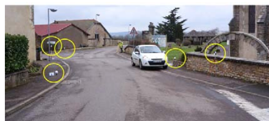
Fig. 11: Reference points for scene georeferencing
