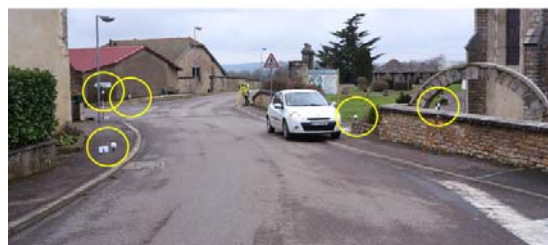
Fig. 11: Reference points for scene georeferencing
