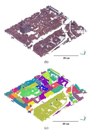
Figure 4. Segmentation into building blocks: (a) ground points; (b) off-ground points; (c) result of block segmentation (one colour per block)
