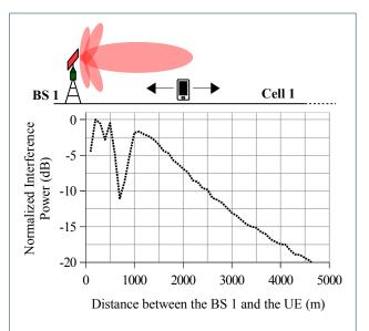
Figure 5 Normalized interference power on the UE side as a function of the distance between the BS 1 and the UE when the MRT precoder is used.
