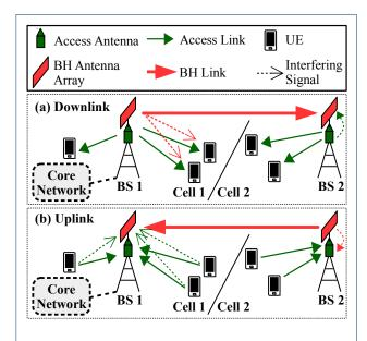
**Figure 2** Description of (a) the downlink and (b) the uplink of the considered in-band wireless BH scenario.
