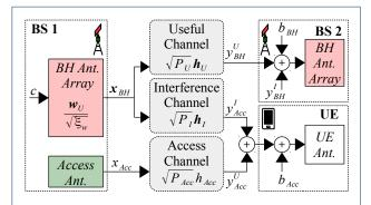
**Figure 3** System model for an in-band wireless BH transmission.
