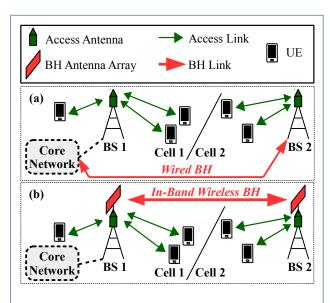
Figure 1 Scenario comparison between (a) a wired BH and (b) an in-band wireless BH.
