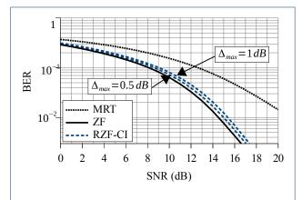
**Figure 6** BER on the UE side as a function of the SNR for the three considered precoding techniques.
