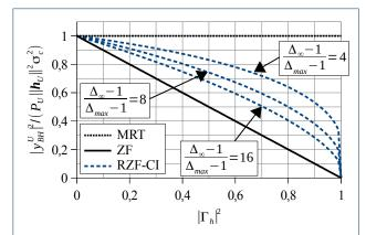
Figure 4 Theoretical normalized received useful power on the BH antenna array of the BS 2 as a function of the correlation factor  $\Gamma_h$ , for the three considered precoding techniques.
