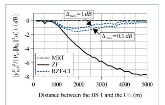
Figure 7 Normalized received useful power on the BH antenna array of the BS 2 as a function of the distance between the BS 1 and the UE for the three considered precoding techniques.
