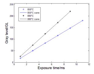
Fig. 3: Relationship between exposure time and gray level of image at the fixed temperature of 850°C and 880°C.
