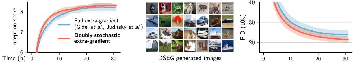
Figure 3: Training curves and samples using doubly-stochastic extrapolation on WGAN-GP, with dataset CIFAR10, for best learning rates. Doubly-stochastic extrapolation allows faster and better training, most notably in term of Fréchet Inception Distance (10k). Curves averaged over 5 runs.
