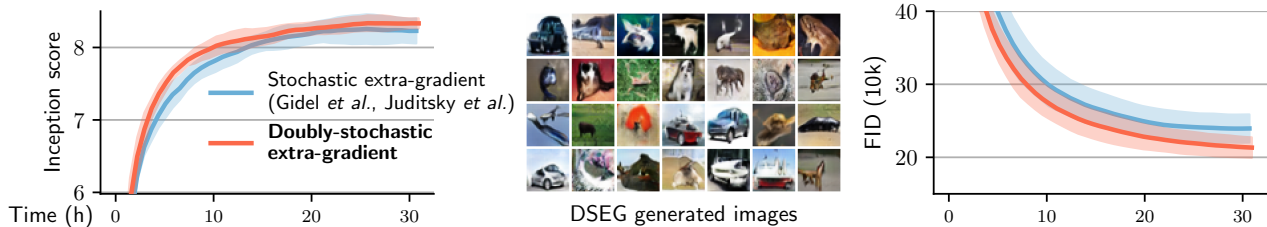
Figure 4. Training curves and samples using doubly-stochastic extrapolation on CIFAR10 with WGAN-GP losses, for the best learning rates. Doubly-stochastic extrapolation allows faster and better training, most notably in term of Fréchet Inception Distance (10k). Curves averaged over 5 runs.
