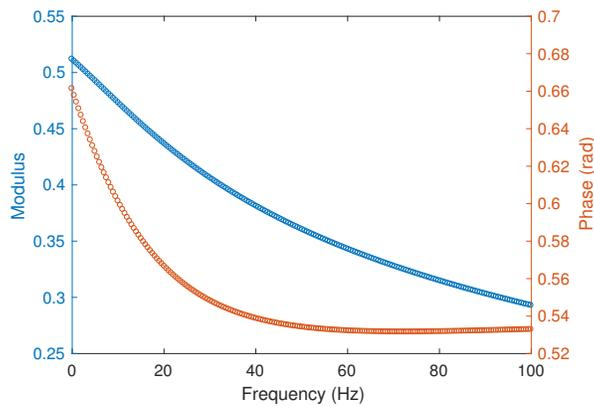
**Figure 4:** Structural damping factor of a railway track
