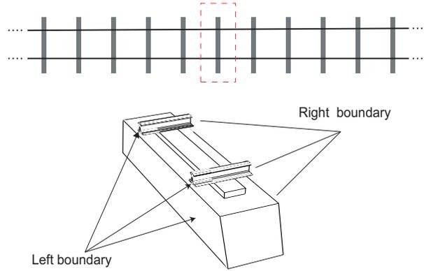
**Figure 1:** Periodic railway track represented by a substructure
