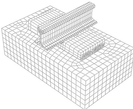
**Figure 6:** Example of a non-ballasted railway track
