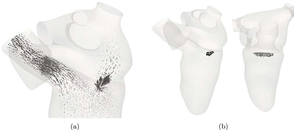
Figure 8: (a) Blood flow during systole for case C09_T3 and (b) associated isovelocity surface in the convergence region, at an aliasing velocity of 25 \text{ cm s}^{-1} , represented as a point cloud.
