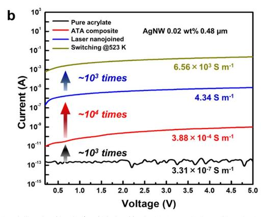
**Figure 1.** (a) Schematic illustration of 3D micro/nanofabrication of functional ATA composites by TPP lithography. (b) I-V curves of barshaped channels fabricated using pure acrylate (black) and ATA composite (red), after laser nanojoining (blue), and thermally treated at 523 K (yellow). The AgNW concentration and length were 0.02 wt% and 0.48  $\mu$ m, respectively.
