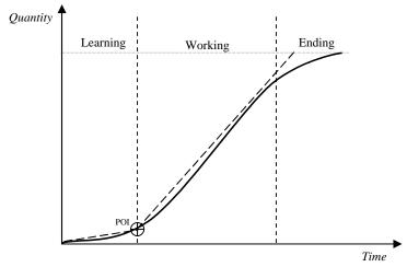
Figure 2: Conventional S-Curve (with straight dashed line)
