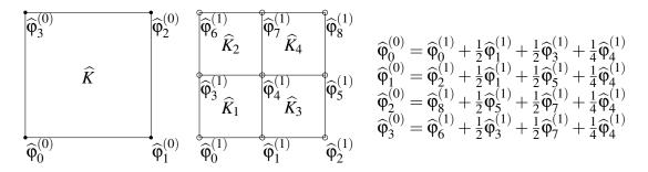
Figure 1: Refinement pattern of a  $\mathbb{Q}_1$  square element and associated refinement equations.
