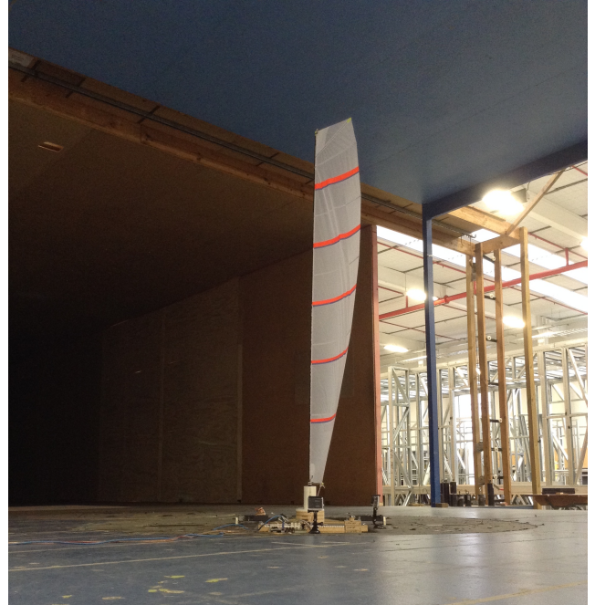
Figure 2: Model mainsail in YRU Twisted Flow Wind Tunnel, University of Auckland
