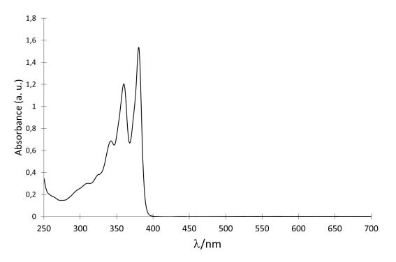
Figure S4. Absorption spectrum of py-NDI recorded in dichloromethane solution.
