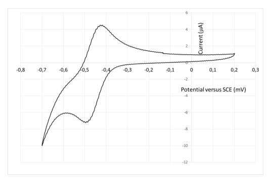
**Figure S2.** Cyclic voltammogram of py-NDI recorded in CH<sub>3</sub>CN with Bu<sub>4</sub>NClO<sub>4</sub> as supporting electrolyte (0.1 M), rate 100 mV/sec.
