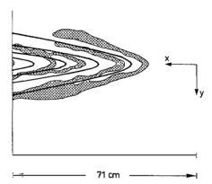
Fig. 5. Phase lines (middle of clear zones) in a horizontal plane z=4.5 cm above the centre of the sphere, located at x, y, z=0, and comparison with linear theory (solid lines). The phase line spacing is  $\lambda/2$
