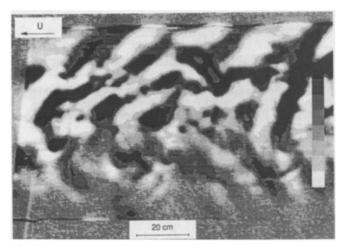
Fig. 7. Visualisation of the phase lines in a horizontal plane z = 12.5 cm above the centre of the obstacle for F = 12.5 and N t = 75.4. Image taken in the big tank 100 cm deep and 300 cm wide. The sphere is moving here from right to left
