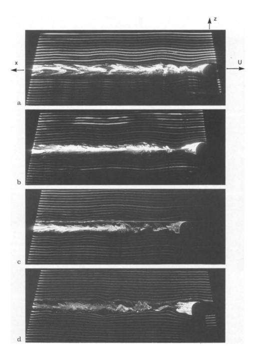
Fig. 2a-d. Visualisation of a vertical section, y=0, of the wake and the internal gravity wave field, predominantly lee waves, in stratified fluid. a, F=1.2, Nt=22.6; b, 1.5, 17.4; c 1.7, 13.7; d, 2.5, 10.2. The non-dimensional times Nt are measured from the center of the sphere and refer to the left hand side of the photographs. The scale is given by the sphere diameter equal to 5 cm. Re is  $3 \cdot 10^3$
